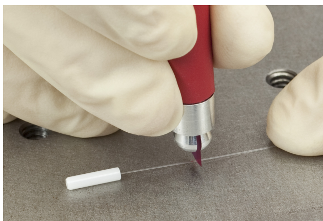
Figure 1: Scribing the Fiber with the S90R Fiber Scribe
