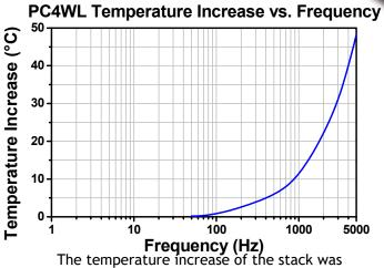
The temperature increase of the stack was measured after applying a sine-wave driving voltage, with maximum and pear-to-peak amplitudes of 150V, at the specified frequency for 10 minutes.
