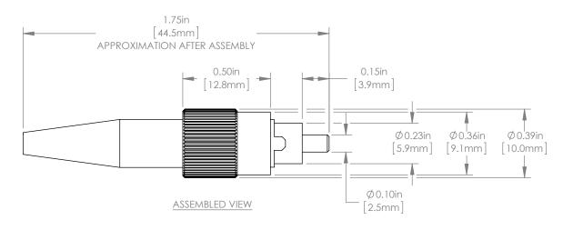
FOR USE WITH SINGLE MODE FIBER ONLY INCLUDED BUT NOT SHOWN PROTECTIVE DUST CAP
