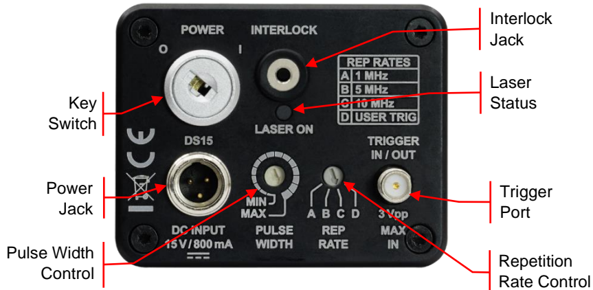
Figure 2 Back Panel of NPLxB Lasers
