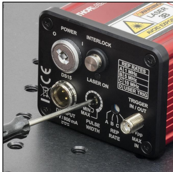
Figure 8 Use the included 2 mm flathead screwdriver to adjust the pulse width and repetition rate controls.
