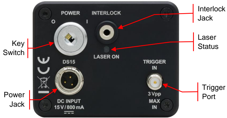
Figure 1 Back Panel of NPLxA Lasers
