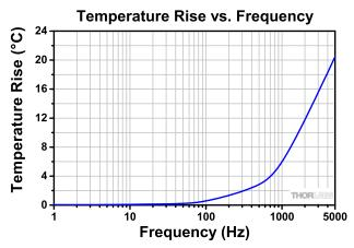
Temperature rises were measured after applying a sine-wave drive voltage ranging from 0 to 150 V at the specified frequency for 10 minutes.
