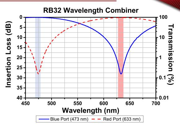
This plot shows the spectral performance of a 2-wavelength combiner. The lines represent the spectral response of each channel, while the colored regions denote the bandwidth around the center wavelengths.
