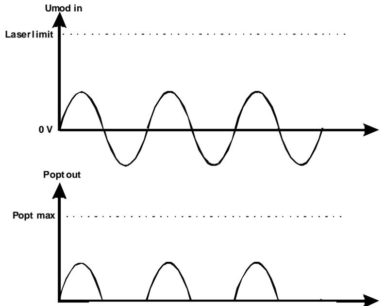
**Figure 13 Power Modulation Clipping.**
