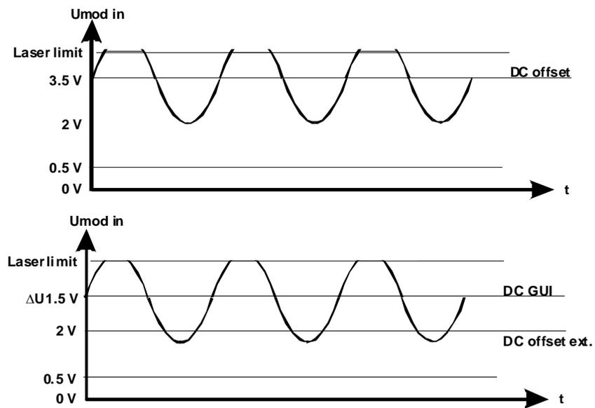
Figure 14 Power Modulation Clipping (offset too high)
