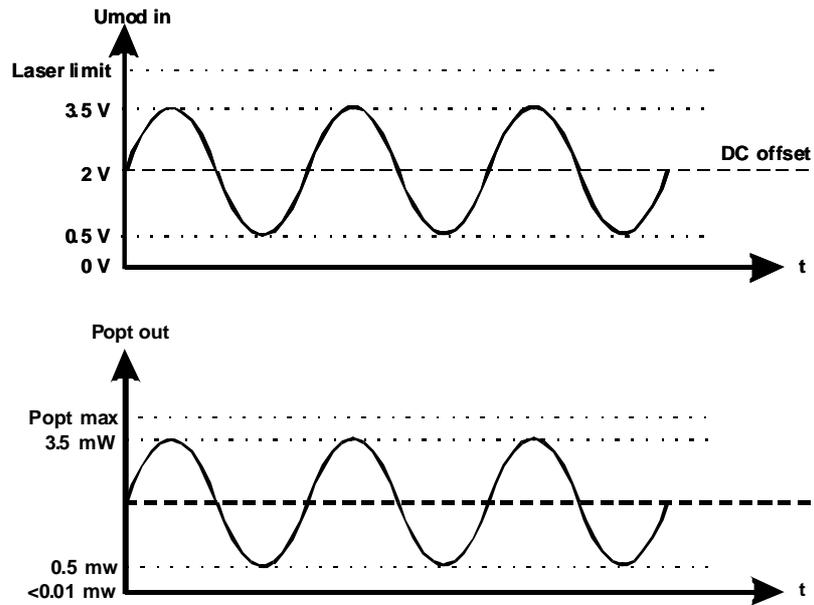
Figure 15 Power Modulation with correct DC offset
