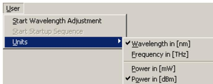
You can select between wavelength in nanometer [nm] or frequency in tera-Hertz [THz] resp. power in milli-Watt [mW] or in decibles above 1 mW [dBm].
