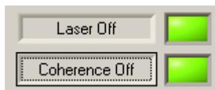
The button marked with 'Laser On' / 'Laser Off' switches the laser output power between the selected output power and a minimum value ( $< -20$  dBm).
