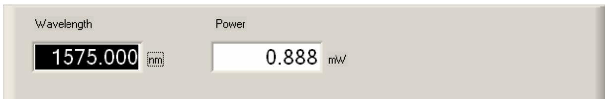
You can enter new numerical values by marking the whole display or single digits with your cursor, then type-in a new value und hit 'Enter'.
