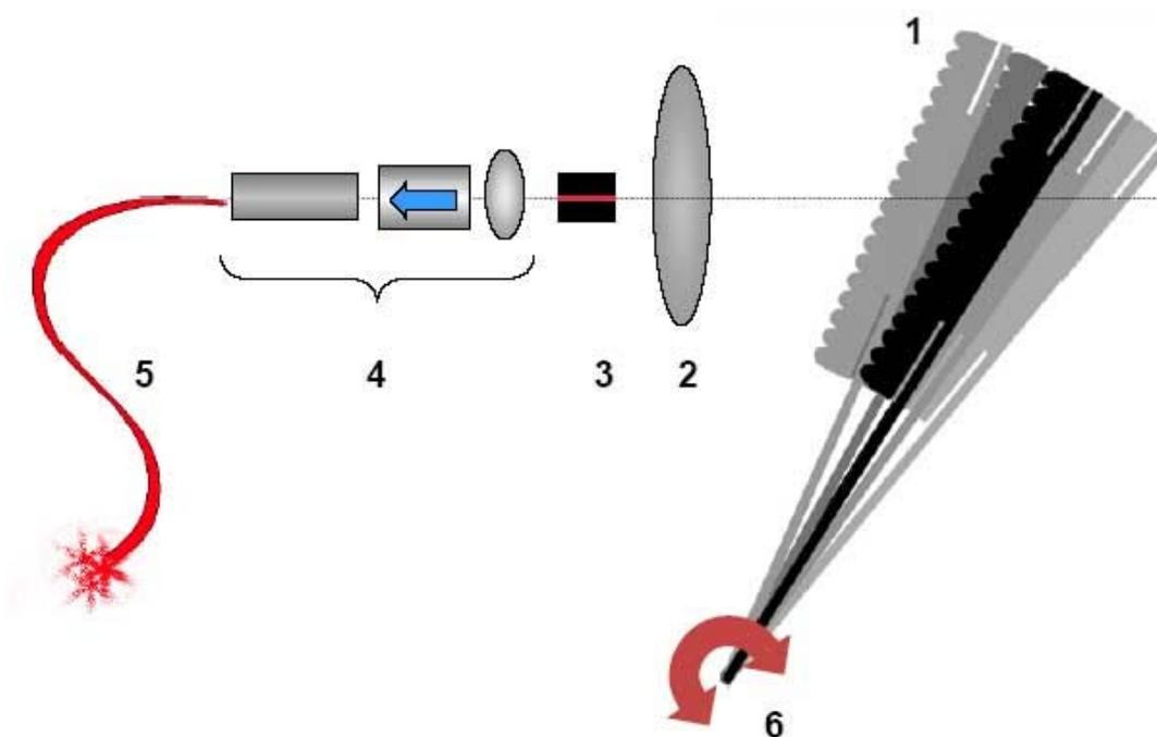
**Figure 2 Principle set-up of the external cavity laser**
