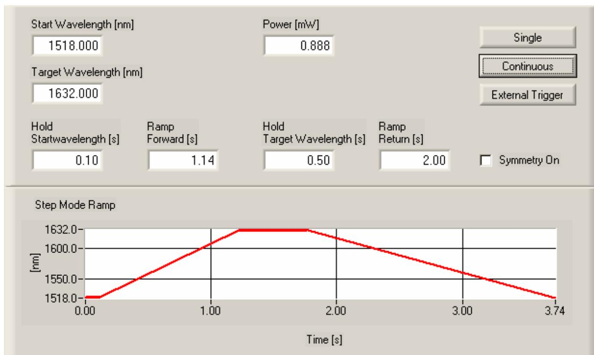
The sweep control panel offers a graphical representation of the sweep, 7 numerical input fields, one checkbox and 3 operating buttons.
