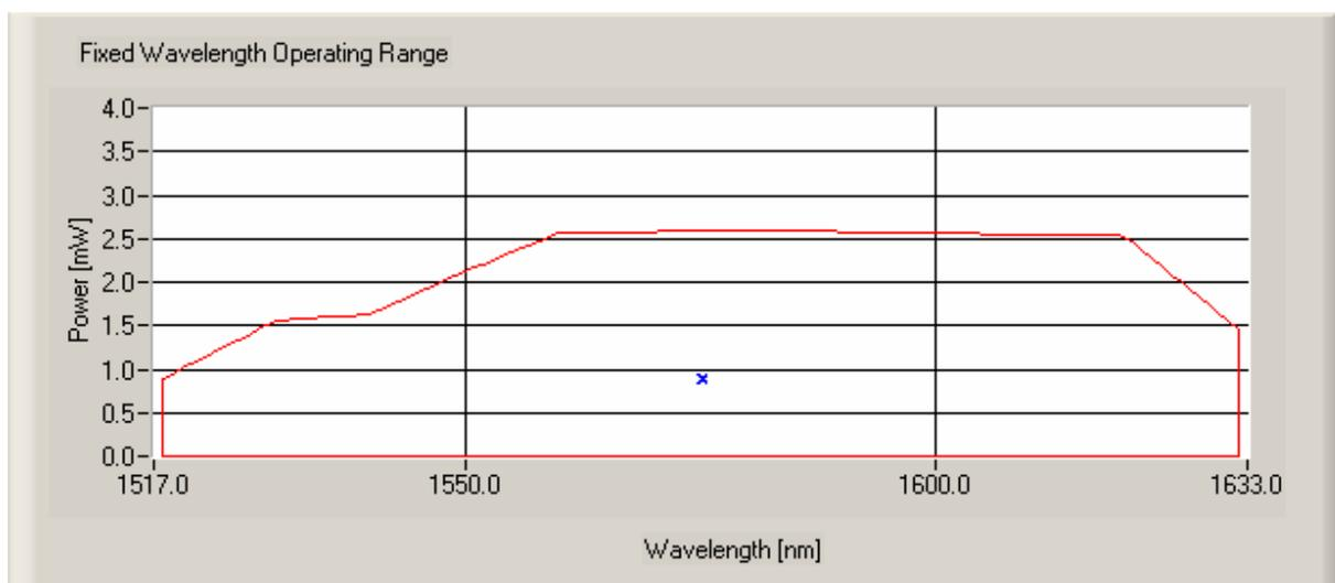
The red surrounded region comprises the operation area, in which no mode hops occur. You can select any wavelength and any power within this graph for mode-hop free operation.
