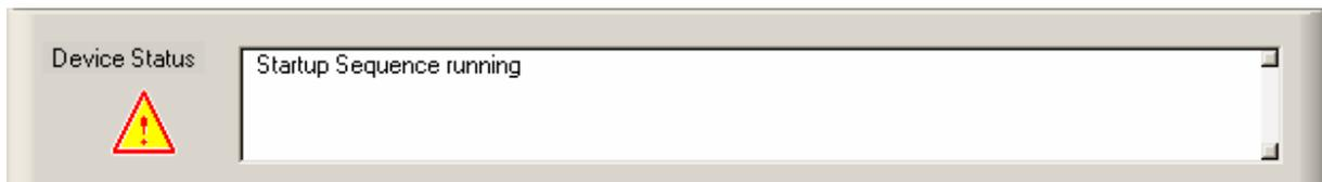
Any status message or warning or occurring error is displayed in the Device Status field. E.g. if the measurement executes the startup sequence after turning it on the first time, the status field shows 'Startup Sequence running'.
