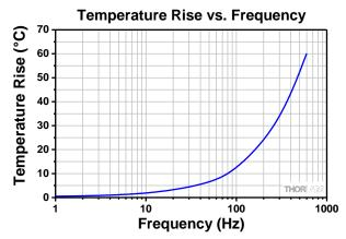
The temperature increase of the stack was measured after applying a sine-wave drive voltage, with maximum and peak-to-peak amplitudes of 75 V, at the specified frequency for 10 minutes.
