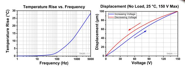
Temperature rises were measured after applying a sine-wave drive voltage ranging from 0 to 150 V at the specified frequency for 10 minutes.
