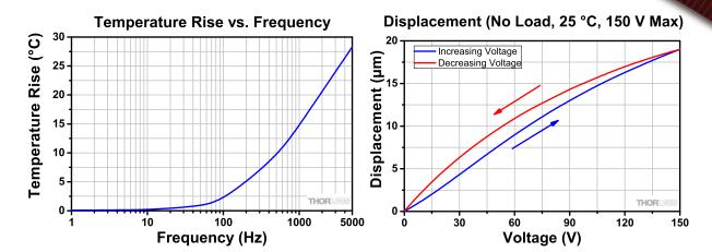
Temperature rises were measured after applying a sine-wave drive voltage ranging from 0 to 150 V at the specified frequency for 10 minutes.
