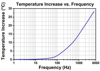
The temperature increase of the chip was measured after applying a sine wave driving voltage, with maximum and peak-to-peak amplitudes of 150 V, at the specified frequency for 10 minutes.
