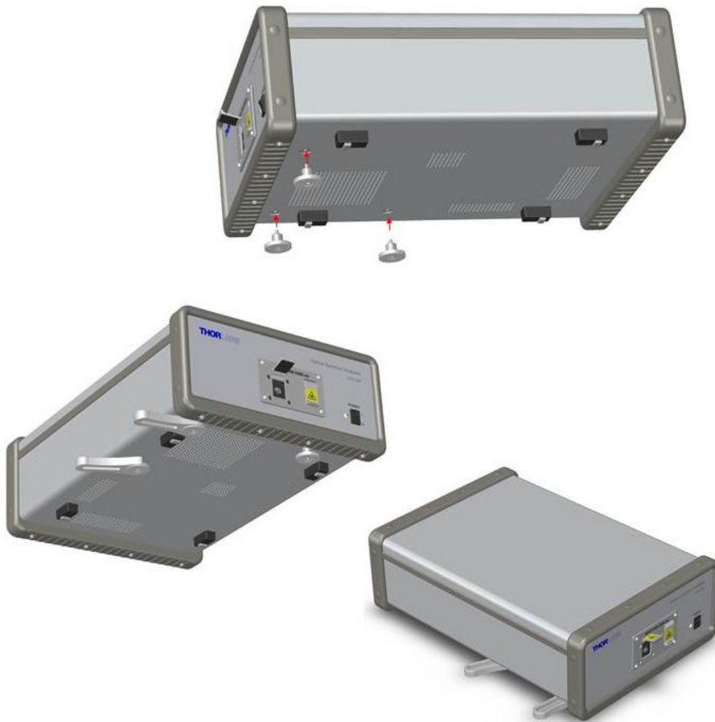
Figure 8 Attach the posts (included) and secure to the breadboard using CF175 clamping forks when using the free space input on the OSA205.
