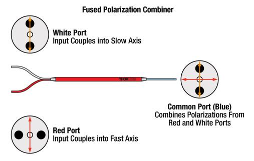
Proper alignment for splitting applications:
