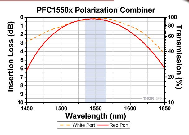
This plot shows the spectral performance of a typical 1550 nm fused fiber polarization combiner. The blue-shaded region denotes the full operating wavelength range. All data was measured without connectors.
