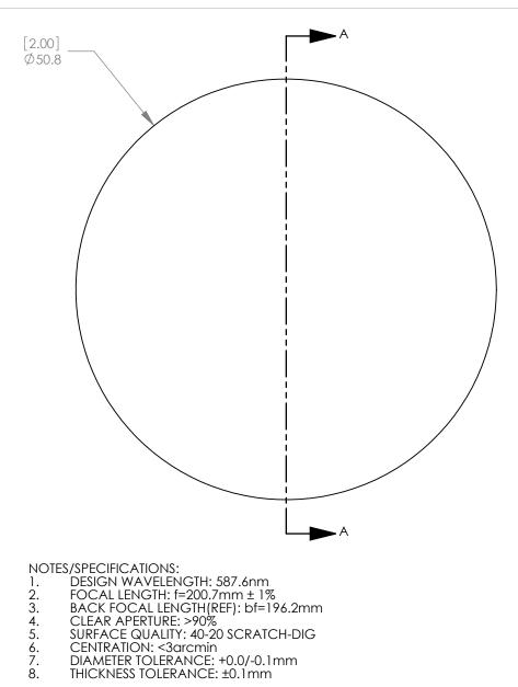
ALL DIMENSIONS ARE IN THE FORM  $\frac{[in]}{mm}$ . THIS DRAWING IS FOR INFORMATION ONLY NOT INTENDED FOR MANUFACTURING
