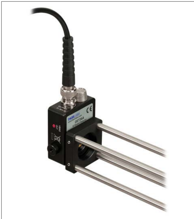
This picture shows a DET series photodetector attached to a CP02 cage plate after removing the SM1T1. The retaining ring from the SM1T1 was used to make the orientation of the detector square with the cage plate.
