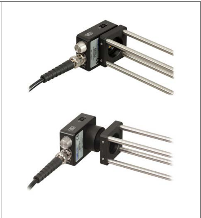
These two pictures show a DET series photodetector in a horizontal configuration. The top picture shows the detector directly coupled to a CP02 cage plate. The bottom picture shows a DET series photodetector attached to a CP02 cage plate using an SM1T2 adapter in addition to the SM1T1 that comes with the PDA series detector.
