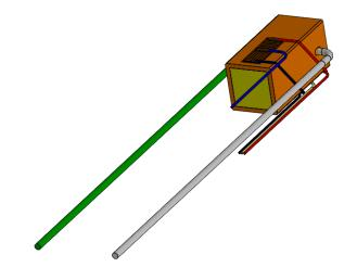
\* All Strain Gauge Wires are 260mm(10.2in) Long with 0.5mm(0.02in) Outer Diameter
