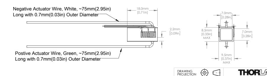
PIEZO ACTUATOR ΥN 15/MAR/21 DRAWN 15/MAR/21 MATERIAL RG APPROVAL N/A FOR INFORMATION ONLY **COPYRIGHT © 2021 BY THORLABS** NOT FOR MANUFACTURING PURPOSES ITEM # VALUES IN PARENTHESIS ARE CALCULATED PC4GQC2 AND MAY CONTAIN ROUNDOFF ERRORS
