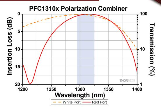
This plot shows the spectral performance of a typical 1310 nm fused fiber polarization combiner. The blueshaded region denotes the full operating wavelength range. All data was measured without connectors.
