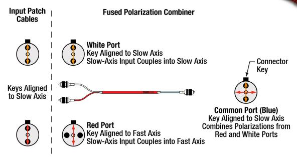
Proper alignment for splitting applications:
