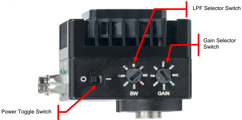
Figure 2 Gain Control, LPF Control, and Power Selector
