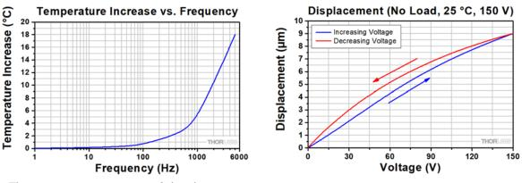
The temperature increase of the chip was measured after applying a sine-wave drive voltage, with maximum and peak-to-peak amplitudes of 150 V, at the specified frequency for 10 minutes.
