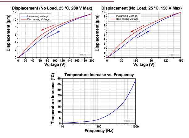
The temperature increase of the chip was measured after applying a sine-wave drive voltage, with maximum and peak-to-peak amplitudes of 200 V, at the specified frequency for 10 minutes.
