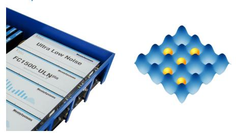
The FC1500-ULN<sup>plus</sup> Ultra Low Noise Optical Frequency Comb brings the system performance to the next level. Additional hardware, optimized components and engineering ingenuity resulted in a perfect flywheel for transferring frequency stability between two or more user-defined frequencies at the 10<sup>-19</sup> level. This exceeds the stability of any optical oscillator demonstrated to date, and transcends the stability requirement for optical clocks.
