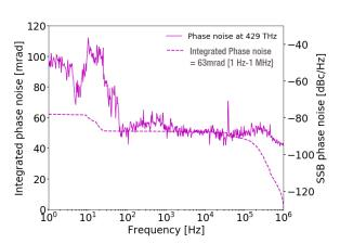
Analysis of the out of loop beat signal between two ULN<sup>plus</sup> combs at the Strontium clock transition frequency:
