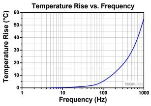
The temperature increase of the stack was measured after applying a sine-wave drive voltage, with maximum and peak-to-peak amplitudes of 150 V, at the specified frequency for 10 minutes.
