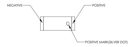
DRAWING PROJECTION  $(\Phi)$ www.thorlabs.com DATE NAME PIEZO ACTUATOR 18/JUN/19 XLIU DRAWN MATERIAL 18/JUN/19 REV APPROVAL SS N/A COPYRIGHT © 2019 BY THORLABS APPROX WEIGHT 0.3 g ITEM # VALUES IN PARENTHESIS ARE CALCULATED AND MAY CONTAIN ROUNDOFF ERRORS PA25FE
