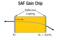
$R_2 = 10\%$  for all models in the SAF series except the SAF1900S, for which  $R_2 = 20\%$ .
