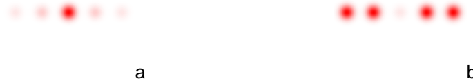
Figure 4 Output beam patterns of the standard contrast OM6N(/M) modulator: (a) powered off or powered on and set to high transmission, (b) powered on and set to low transmission. Only the central beam passes through the output aperture when the beam is properly aligned.
