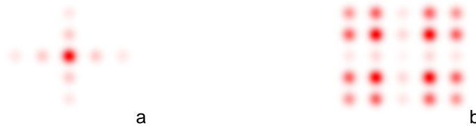
Figure 5 Output beam patterns of the high contrast OM6NH(/M) and OM6ENH(/M) modulators: (a) powered off or powered on and set to high transmission, (b) powered on and set to low transmission. Only the central beam passes through the output aperture when the beam is properly aligned.
