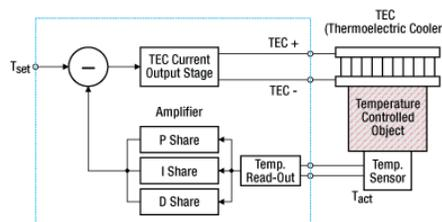
TEC Driver Integrated into a Circuit with a TEC and Temperature Sensor
