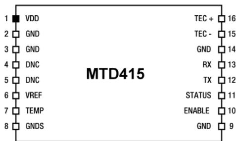
These pin assignments correspond to viewing the driver from the top when the engraving on the driver is right-side up.
