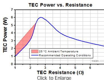
The maximum output power of 6 W can be delivered into a load resistance of 2.66 Ω under the recommended operating conditions. The maximum output power at lower than 2.66 Ω load resistance (shaded range) depends on environmental conditions.
