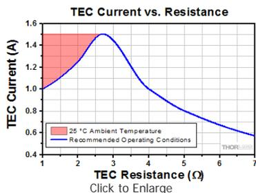
The maximum TEC current of 1.5 A can be delivered into a load resistance of 2.66 Ω under the recommended operating conditions. At a higher load resistance, the maximum output current drops due to the limit of the compliance voltage. The maximum output current at lower than 2.66 Ω load resistance (shaded range) depends on environmental conditions.
