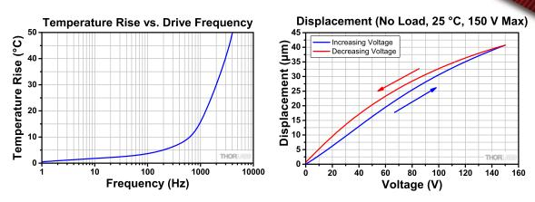
These temperature rises were measured after applying a sine-wave drive voltage ranging from 0 to 150 V at the specified frequency for 10 minutes.
