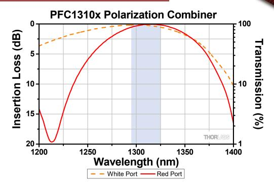
This plot shows the spectral performance of a typical 1310 nm fused fiber polarization combiner. The blueshaded region denotes the full operating wavelength range. All data was measured without connectors.
