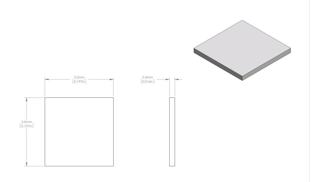
THORLABS www.thorlabs.com DRAWING PROJECTION DATE NAME 5.0X5.0X0.4MM END PLATE JAN/14/15 YWA DRAWN MATERIAL REV A SRU JAN/14/15 APPROVAL AL2O3 COPYRIGHT © 2015 BY THORLABS APPROX WEIGHT ITEM # VALUES IN PARENTHESIS ARE CALCULATED 0.09 g PKFEP4 AND MAY CONTAIN ROUNDOFF ERRORS
