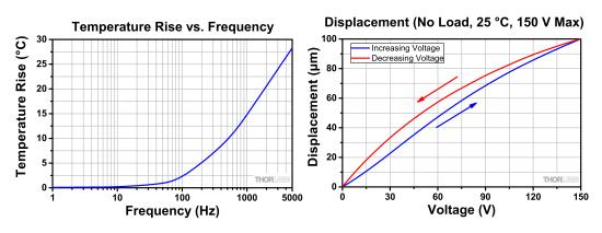
Temperature rises were measured after applying a sinewave drive voltage ranging from 0 to 150 V at the specified frequency for 10 minutes.
