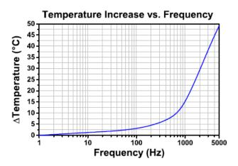
The temperature increase of the chip was measured after applying a sine-wave drive voltage, with maximum and peak-to-peak amplitudes of 150 V, at the specified frequency for minutes.
