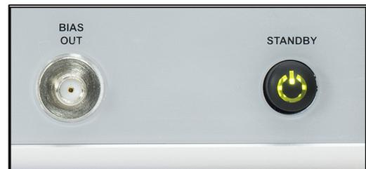
Turn on the MBX by pressing the amber standby button on the front panel until it turns green (about 1 sec) to indicate the unit is fully on. The touchscreen display will come up with a boot screen for about 5 seconds and then go to the home page. The unit will initialize in the factory default state with all functions OFF.
