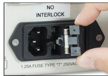
5. Investigate the fuse. This can be done with a simple continuity check. If in doubt, replace the fuse. A spare fuse is stored in the fuse holder. Additional replacement fuses can be purchased from Thorlabs. **Always use fuses of the same type as the original.**
