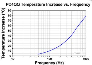
The temperature increase of the stack was measured after applying a sine-wave driving voltage, with maximum peak-to-peak amplitudes of 150 V, at the specified frequency for 10 minutes.
