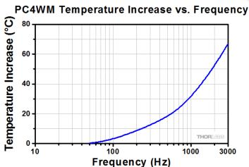
The temperature increase of the stack was measured after applying a sine-wave driving voltage, with maximum and peak-to-peak amplitudes of 150 V, at the specified frequency for 10 minutes.
