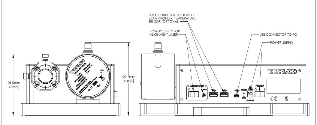
DRAWING PROJECTION THORLABS www.thorlabs.com  $\bigcirc$ NAME DATE M<sup>2</sup> MEASUREMENT SYSTEM WITH BP209-IR2/M, 900-2700nm, METRIC Hit. 12/JUN/17 DRAWN RR 12/JUN/17 APPROVAL N/A COPYRIGHT © 2017 BY THORLABS APPROX WEIGHT ITEM # VALUES IN PARENTHESIS ARE CALCULATED M2MS-BP209IR2/M 4.6 kg
