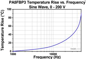
This test was conducted by applying a sine-wave driving voltage, 0 V to 200 V, at the specified frequency for 10 min, at room temperature without cooling. With lower maximum voltage and extra cooling measures, the working frequency can be higher, but the temperature of the device should be kept <130 °C.
