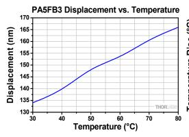
The displacement of the stack was measured after heating to the set temperature for 10 minutes.
