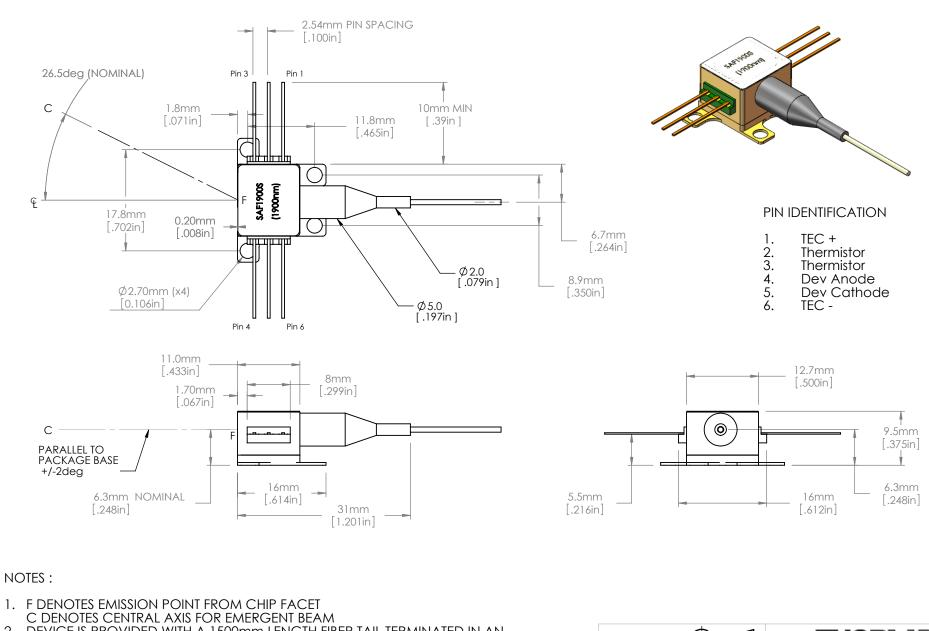
DEVICE IS PROVIDED WITH A 1500mm LENGTH FIBER TAIL TERMINATED IN AN FC/APC CONNECTOR; THE FIBER IS THORLABS SM2000 TYPE PROTECTED BY 900um DIAMETER LOOSE TUBE
