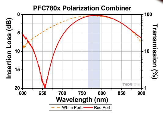
This plot shows the spectral performance of a typical 780 nm fused fiber polarization combiner. The blue-shaded region denotes the full operating wavelength range. All data was measured without connectors.
