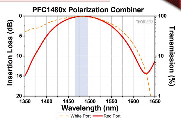
This plot shows the spectral performance of a typical 1480 nm fused fiber polarization combiner. The blue-shaded region denotes the full operating wavelength range. All data were measured without connectors.
