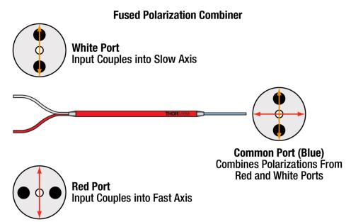
Proper alignment for splitting applications:
