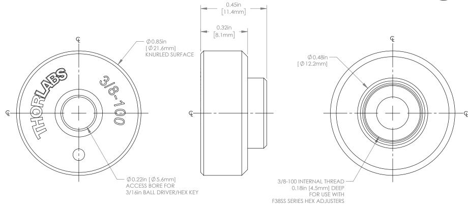
DRAWING PROJECTION THORLABS www.thorlabs.com  $\bigoplus$ NAME DATE 3/8-100 LARGE ADJUSTER KNOB 06/NOV/19  $\mathsf{AK}$ DRAWN 07/NOV/19 MATERIAL ANODIZED ALUMINUM APPROVAL ZΜ REV COPYRIGHT © 2019 BY THORLABS APPROX WEIGHT ITEM # VALUES IN PARENTHESIS ARE CALCULATED AND MAY CONTAIN ROUNDOFF ERRORS F38SSK1L 7.5 g
