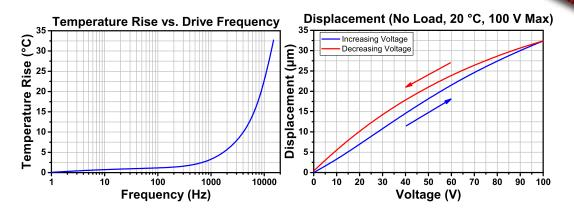
These temperature rises were measured after applying a sine-wave drive voltage ranging from 0 to 100 V at the specified frequency for 10 minutes.
