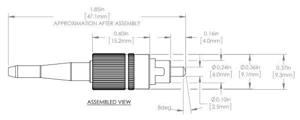
FOR USE WITH SINGLE MODE FIBER AND 900  $\mu m$  TUBING ONLY INCLUDED BUT NOT SHOWN
