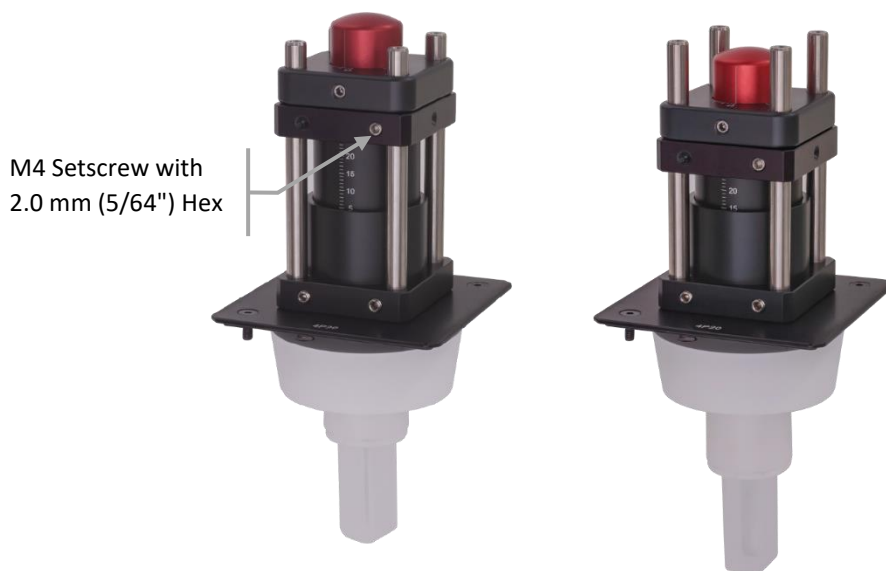
Figure 4 Loosen the M4 Setscrew to Raise and Lower the Cuvette
