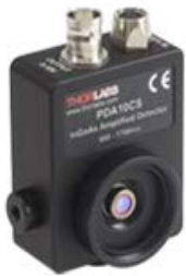
PDA10CS Switchable Gain 17 MHz Max Bandwidth
