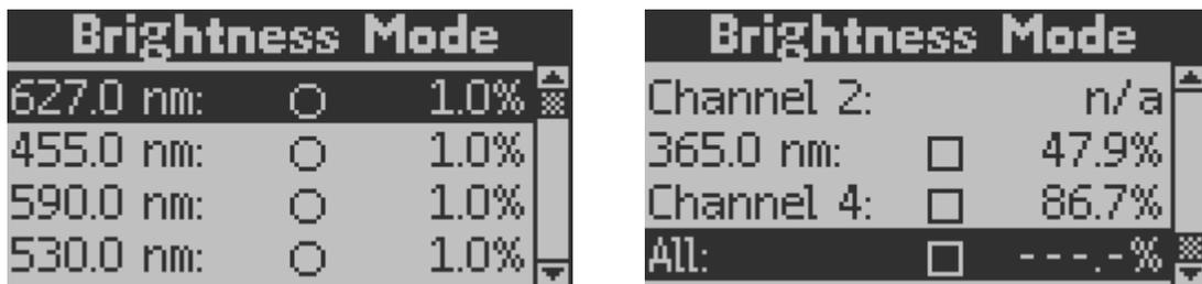
**Figure 9 Brightness Mode: Channel Selection**
