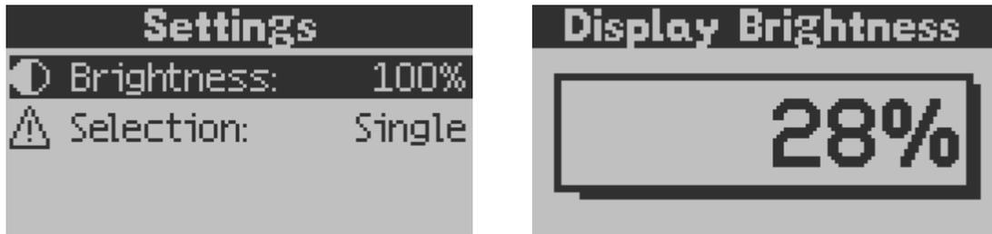
**Figure 17** Display Brightness Setting
