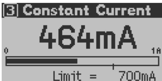
**Figure 8 Constant Current Mode: Current Setting**
