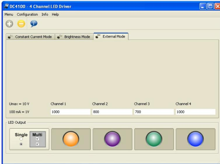
Figure 26 The External Control Mode
