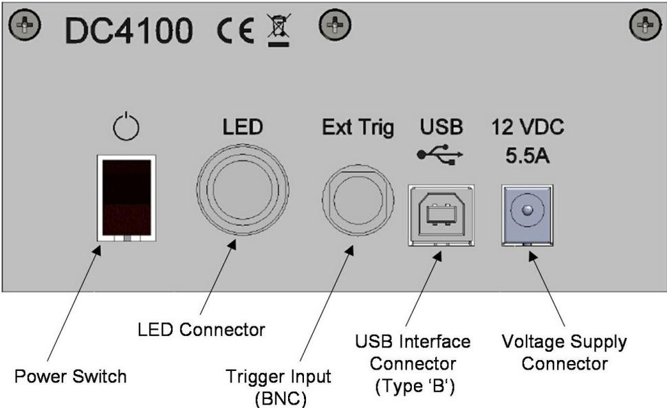
Figure 3 Operating Elements on the Rear Panel
