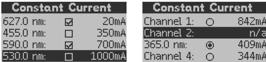
**Figure 7 Constant Current Mode: Channel Selection**
