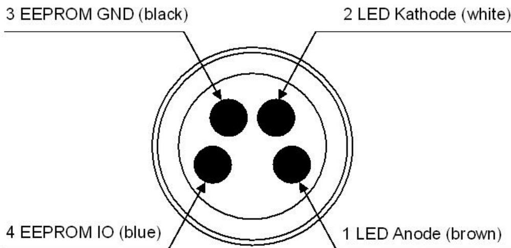
**Figure 32** Female Connector of the DC4100-HUB
