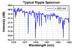
The sharp dips in the ripple spectrum are mostly caused by water absorption in the measurement setup.
