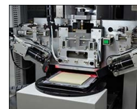
Click to Enlarge Dicing the PZT Block into Individual Elements
