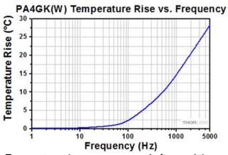
Temperature rises were measured after applying a sine-wave drive voltage ranging from 0 to 150 V at the specified frequency for 10 minutes.
