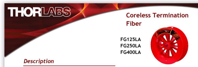
These coreless silica termination fibers can be spliced to the ends of standard fiber to reduce back reflections or prevent damage to the fiber end face. A return loss of greater than 65 dB is achieved by splicing 0.25 m of coreless fiber to the desired component.
