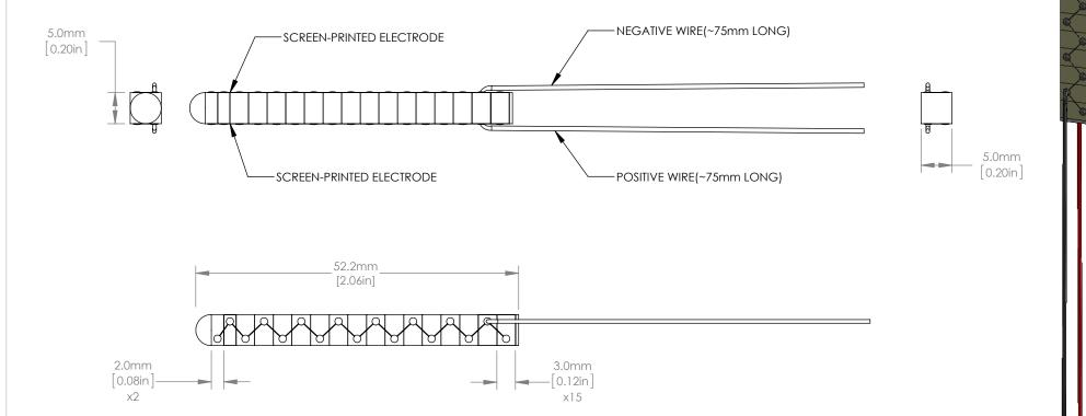
DATE NAME PIEZO ACTUATOR STACK YWA JUN/12/15 DRAWN MATERIAL JUN/12/15 APPROVAL SS N/A COPYRIGHT © 2015 BY THORLABS ITEM # VALUES IN PARENTHESIS ARE CALCULATED AND MAY CONTAIN ROUNDOFF ERRORS
